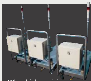
When high-precision ultrasonic sensor detects oil leakage, it shuts off the power and issue an abnormal signal
